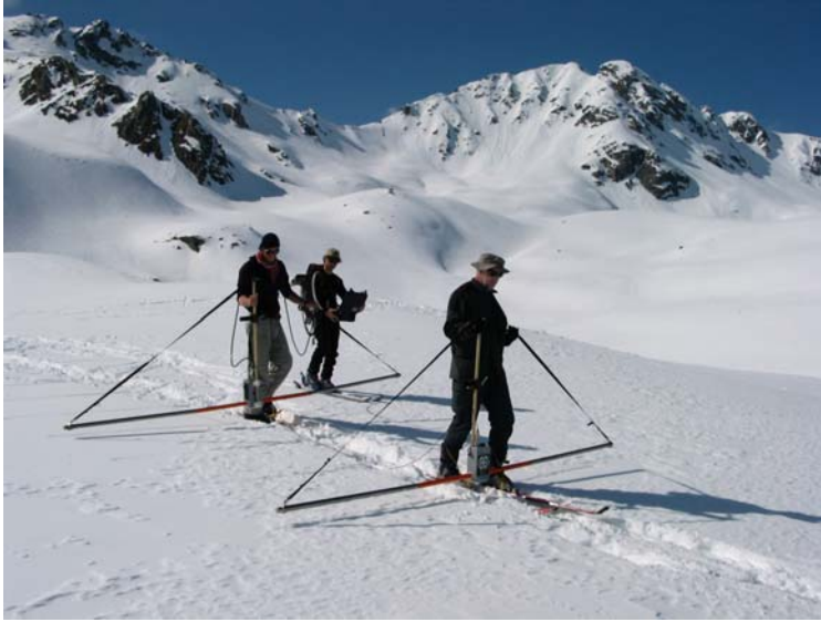
Ground Penetrating Surveying on a rock glacier using a GSSI SIR 2000 equipped with a multiple low frequency antenna with a centre frequency Of 35 MHz. Best results on rock glaciers are achieved when measurements are carried out during winter when the rock glacier is covered with a thick snow cover.
