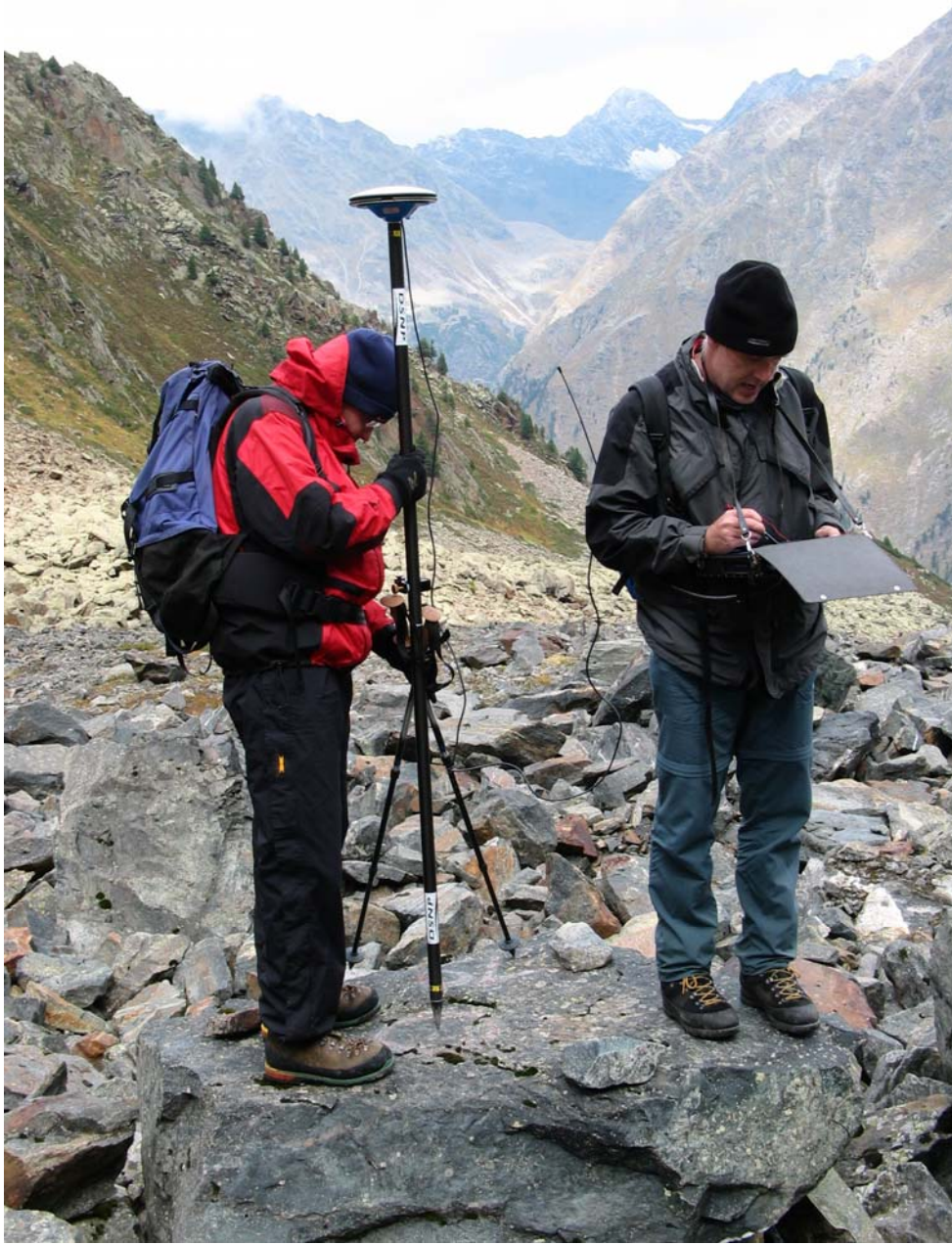
Rover used to measure the survey markers on the Reichenkar rock glacier by real time kinematics (RTK)
