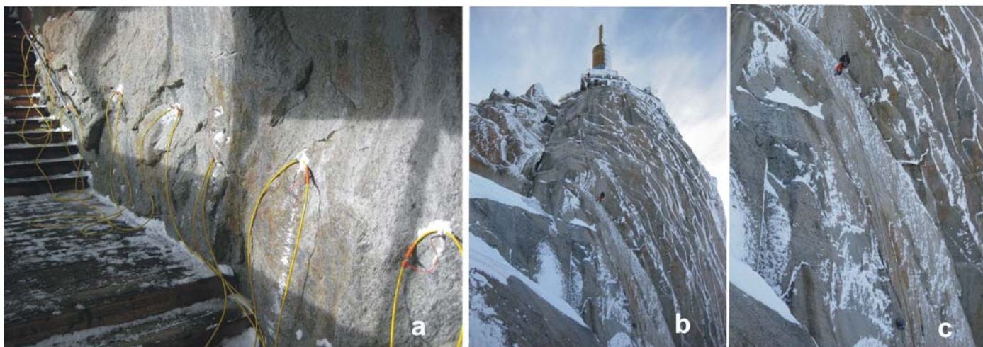
Electrode array along the Piton Nord (Aiguille du Midi); b and c) Installation of electrode array at the Piton Central (Aiguille du Midi, summit 3842 m a.s.l.) in December 2008 (climber: L. Ravel). Photos M. Krautblatter
