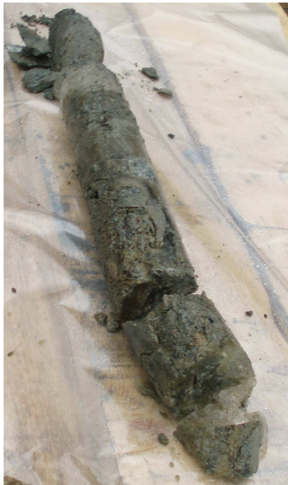
Fig. 8: Frozen core (mixture of debris and ice), Lazaun 1
