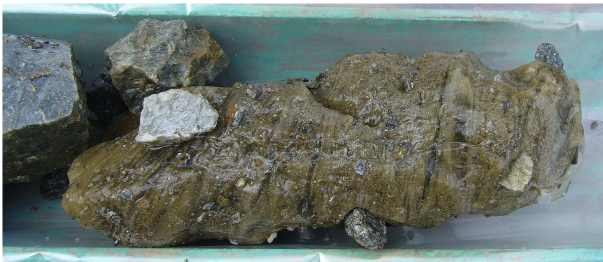
Fig. 9: Ice core composed of banded ice and small clasts
