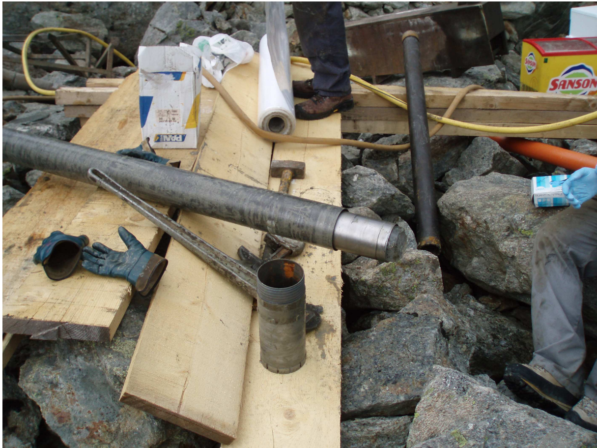
Fig. 7: Drill pipe with ice core, Lazaun 1
